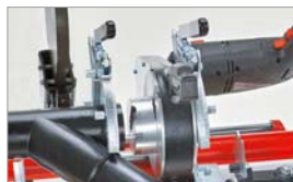
Trimmer attachment (No. 54040) (special accessories)
