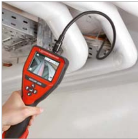
Inspection of hollow spaces
