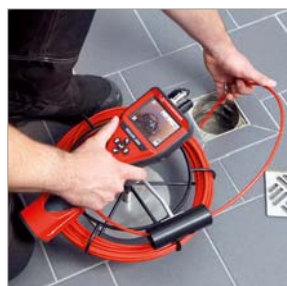
Inspection from floor drains
