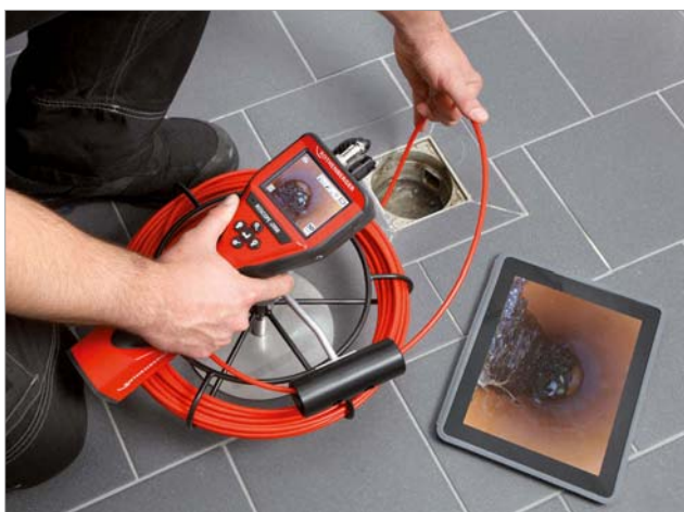
Inspection of basin drains
