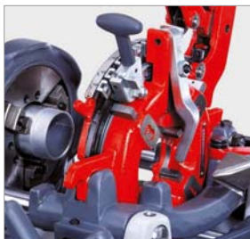
Automatic die head with integrated oil supply
