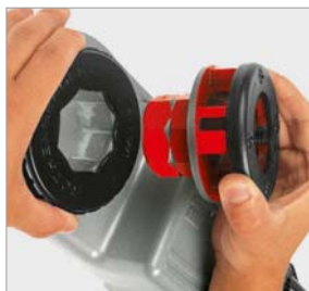
Easy insertion of the die heads
